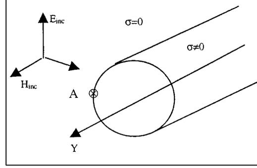
Fig. 3. Plane wave on a conducting cylinder.
