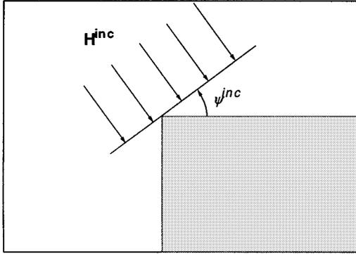
Fig. 3. Diffraction of the plane wave by conducting edge.
