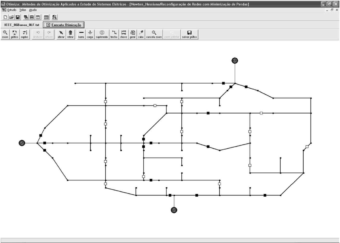
Fig. 2. Ninety-six-branch, 28-switch validation system.
