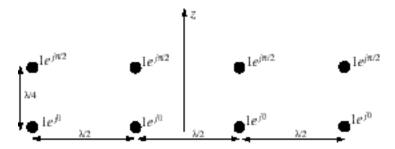
**Solution:** View this two dimensional array as a one dimensional array of four antennas where each antenna is a two element (vertical) array. Then, we first calculate the radiation pattern of the two element array and multiply this by the array factor of a four element linear array.
